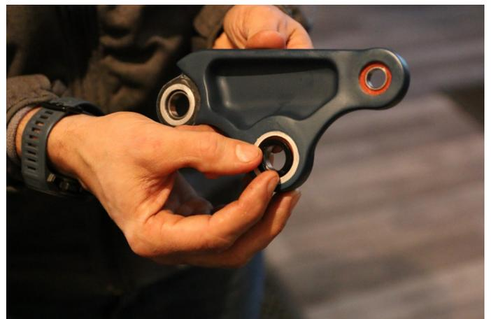
**Step 28 continued:** Grease the shafts of the rocker pivot and place blue Loctite on the threads of the rocker pivot.
