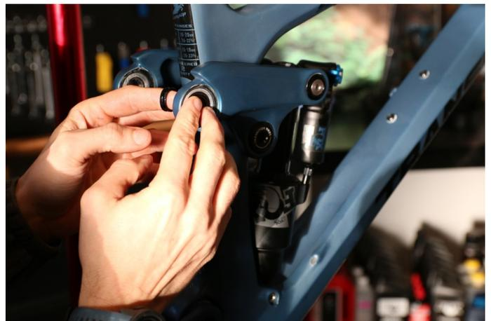
**Step 31 continued:** It's helpful to pinch the bearing spacers when sliding the seat stay onto the rocker.
