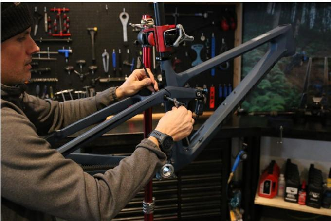
**Step 4:** Repeat step two for the seat stay / rocker junction. Be careful to be mindful with the bearing spacers.
