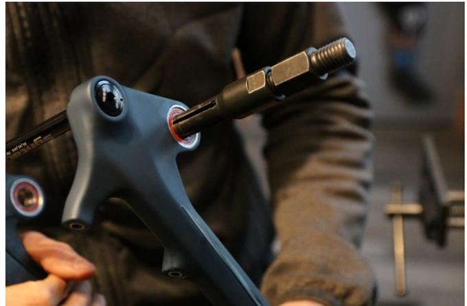
**Step 16 continued:** Connect the slide hammer and move the slide away from the bearing while doing your best to stabilize the seat stay.
