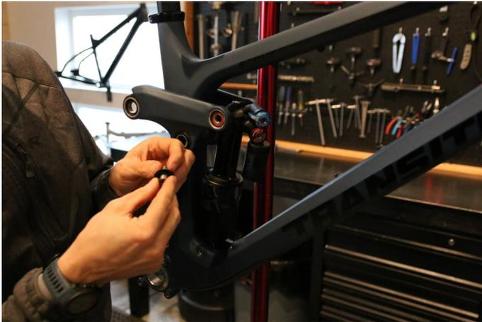
**Step 9 continued:** See small trunion spacers below. The rocker is a two piece rocker, allowing you to remove one side at a time if you'd like.
