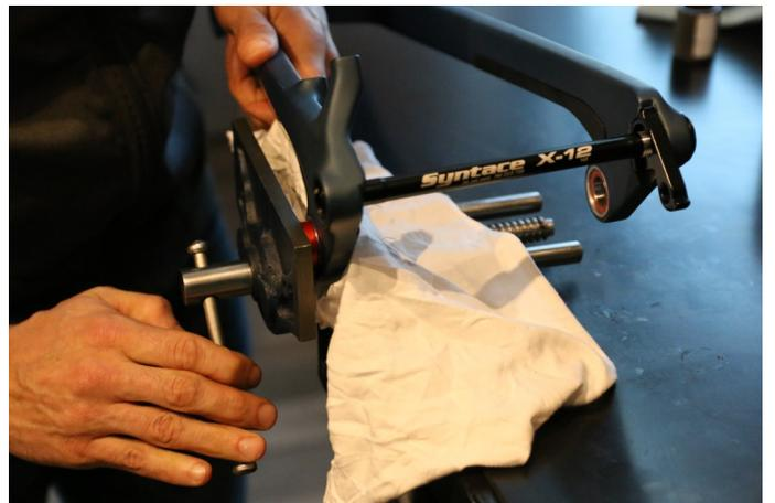
**Step 21:** Install the rocker bearings (3802x2, 6900x2, 6902x2), make sure to grease all bearing seats before installing the bearings. When placing the rocker in the vise be careful to not scratch it.
