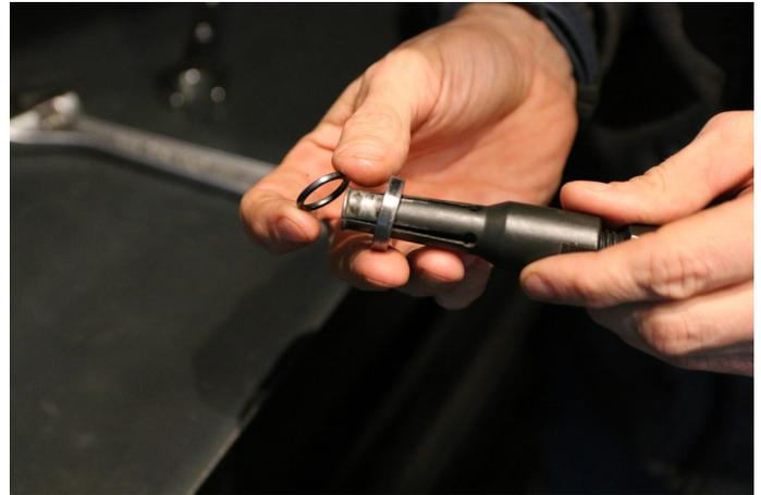
**Step 17:** Now that you've removed the outer bearing, you can push the inner bearing out. Then repeat steps 15-17 on the other side of the seat stay.
