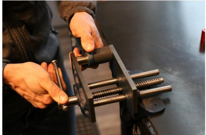
**Step 15 continued:** Make a note of the bearings and snap rings orientation, there are three different sizes.
