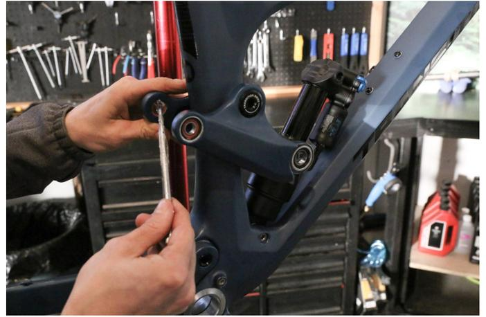
**Step 30 continued:** Add a touch of Loctite to the threads located on the trunion mount.
