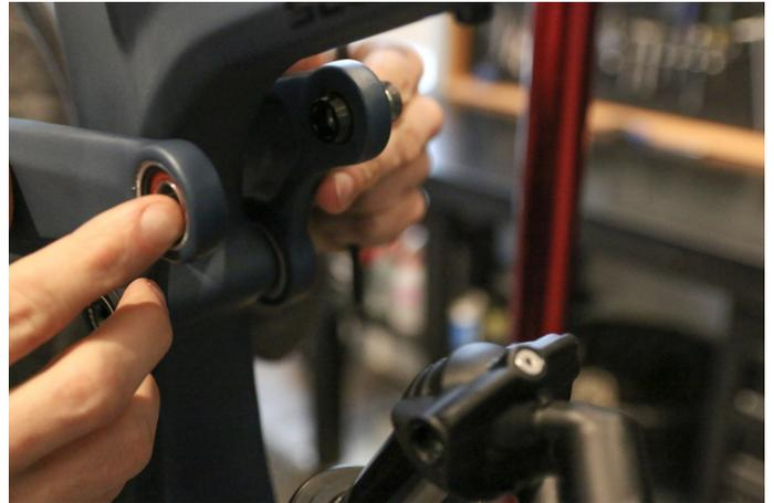
**Step 10:** Remove the lower shock bolt and shock from the frame. You'll need 2, 5mm allen wrenches.
