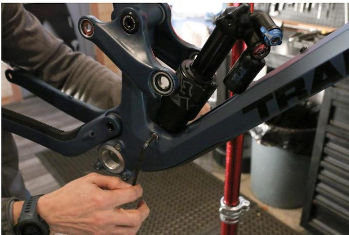
**Step 11:** Remove the upper pivot and then the rocker. You'll need 2, 8mm allen wrenches. Watch for the bearings spacers located on the inside of the rocker.
