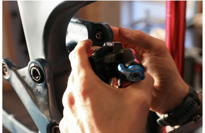
**Step 30 continued:** Snug down the shock bolts using a 5mm allen wrench. Once snug use a torque wrench and tighten to 12Nm. Now you can torque the lower shock bolt to 10Nm.
