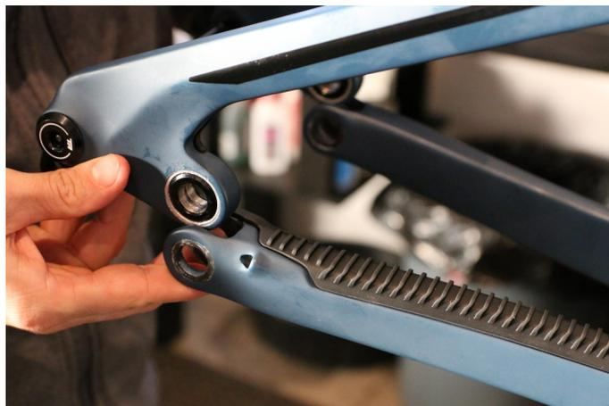
**Step 31 continued:** Grease all the pivot axles and install them. The shorter axles are for the rocker/seat stay junction and the longer ones are for the seat stay/chain stay junction.
