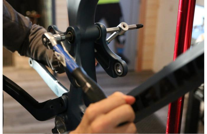
**Step 29:** Install the shock, installing the lower shock bolt first. Make sure to grease the shaft and add blue Loctite to the inside of the female end. You'll need two 5mm allen wrenches to snug the bolt down. Torque to spec (10Nm) after the upper shock bolts are installed.
