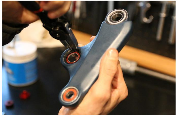
**Step 23:** Grease the main pivot bearing seats and install the main pivot bearings (6903). Install one at a time and make sure to put in the bearing spacer before installing the second bearing.
