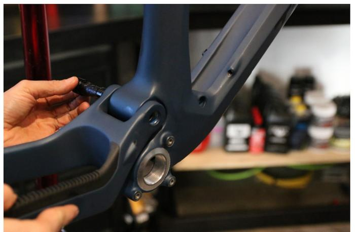
**Step 26 continued:** Snug the main pivot with an 8mm allen wrench. Then use a torque wrench and tighten to 19Nm.
