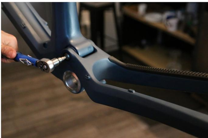
**Step 28:** Install the rocker and rocker pivot, but first add dab of grease to the inside of the center bearing to help hold the bearing spacer in place during installation.
