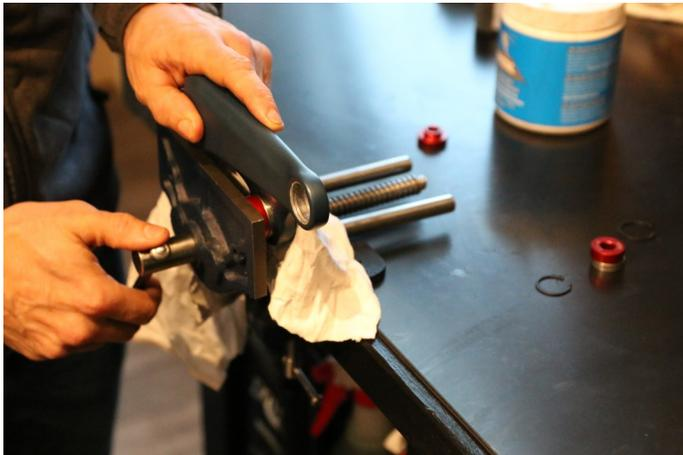
**Step 22:** After you've installed the bearings go ahead and install the snap rings using your snap ring pliers. Make sure to take note of the different sizes and orientation.
