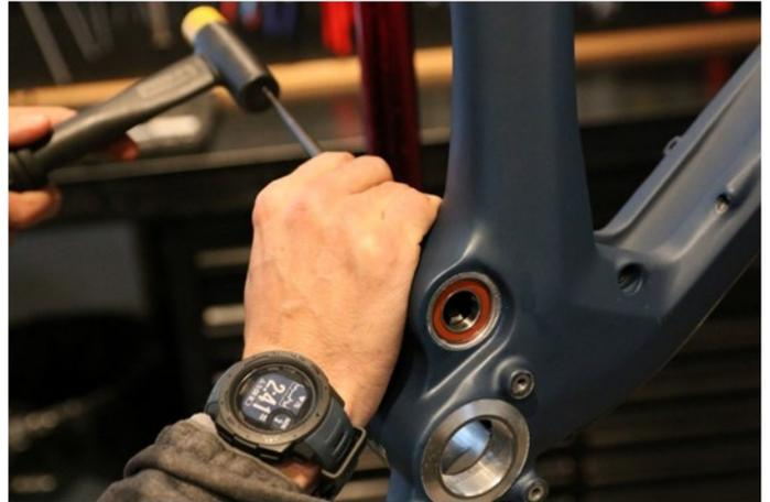
**Step 13:** Remove the spacer and tap the remaining main pivot bearing out of the frame. Making sure to alternate where you're placing the punch to ensure a straight and smooth removal.
