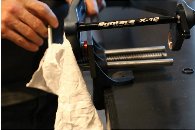
**Step 19:** Insert the bearing spacer and add grease to the bearing seat.
