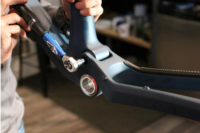
**Step 27:** Install the main pivot screw, spacer, and taper nut. Apply grease to the main pivot taper nut, and blue Loctite on the threads of the main screw after the taper nut is installed.
