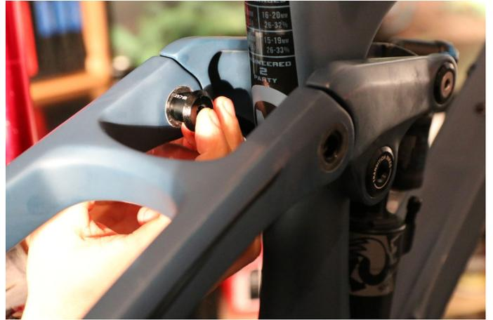
**Step 31 continued:** Add a small amount of grease to the outsides of all four bearings located towards the rear of the seat stay to help keep the bearing shields stay in place. Then carefully slide the chain stay over the seat stay. Be mindful to not pull up on the seat stay as it will potentially damage the seat stay / rocker junction.
