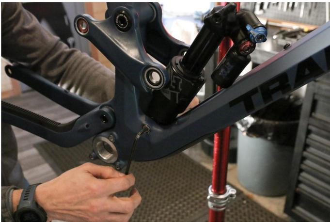
**Step 30:** Install the upper shock bolts. First add a dab of grease to the inside and outside of both forward rocker bearings.
