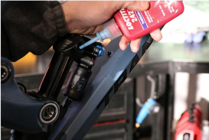
**Step 30 continued:** Attach trunion shock bolt, washer, and tapered spacers. The grease should help hold the spacers in place. It's helpful to insert the shock bolt just far enough to make contact with the spacer.
