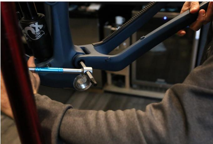
**Step 8:** Remove main pivot bearing shields, make note of orientation of the cover. The smooth side faces away from the bearing and the ridged side faces the bearing.
