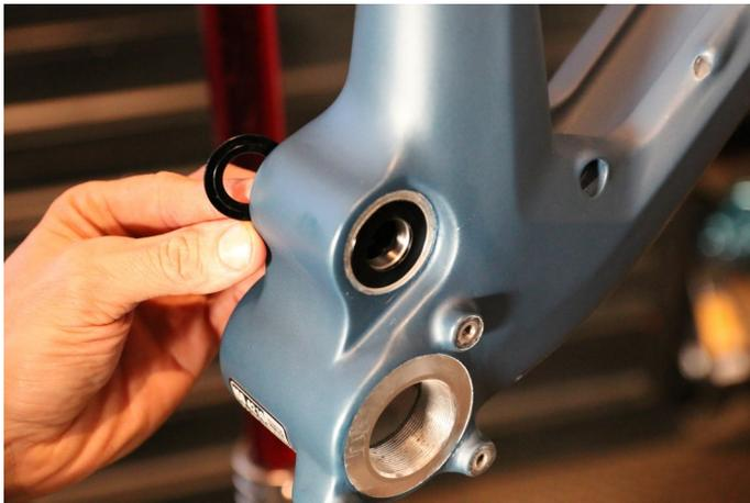
**Step 25:** Place a few drops of blue Loctite on the threads of the chain stay where you the main pivot threads into.
