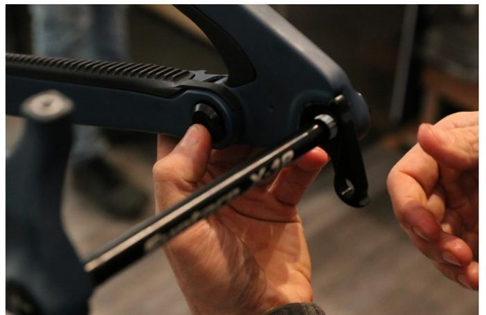
**Step 31 continued:** Add a little bit of Loctite to the female ends of the upper seat stay pivots. Use a 5mm and a 6mm allen wrench to snug them down. Then use a torque wrench and tighten to 12Nm.
