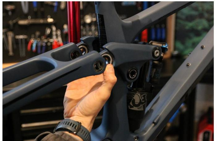
**Step 5:** Remove the cable guide from the main pivot by lightly pulling on it.
