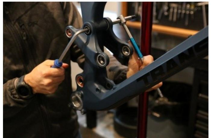
**Step 11 continued:** Below you can see the rocker is two pieces, make sure to account for the spacers located on the inside of the rocker where it mounts to the frame. Now that you have all the pivot hardware removed and accounted for it's time to start removing the bearings.
