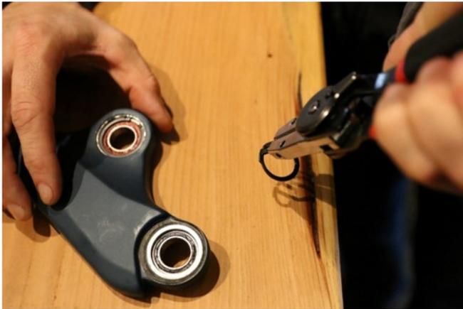
**Step 15:** Remove the rocker bearings. Here you can see the use of the PVC pipe. It allows us to push the bearings out of the rocker. Repeat this procedure for the remaining 5 rocker bearings.
