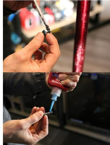
**Step 27 continued:** Snug down the main pivot screw with a 5mm allen wrench. Once snug use a torque wrench to tighten to 10Nm.
