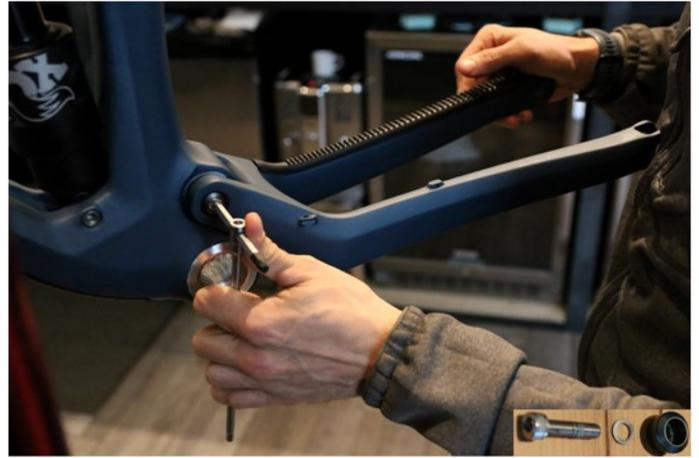
**Step 7:** Remove the main pivot from the frame by using an 8mm allen wrench.
