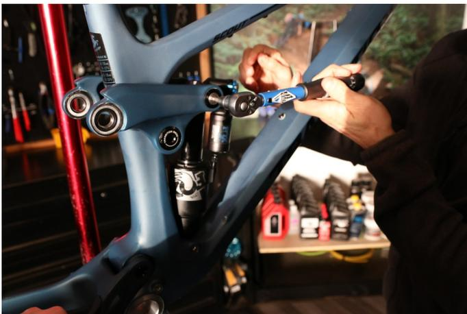
**Step 31:** Attach the seat stay to the rocker, but first lightly grease the seat stay / rocker junction bearings and attach bearing spacers.
