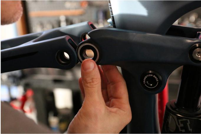
**Step 31 continued:** Slide the seat stay / rocker pivot axles into place. Make sure to add a little grease to the axle body.
