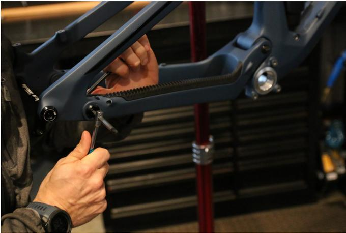
**Step 2:** Slowly and carefully push up on the chain stay, placing your fingers over the bearing spacers to help from losing them. Once detached remove the spacers.
