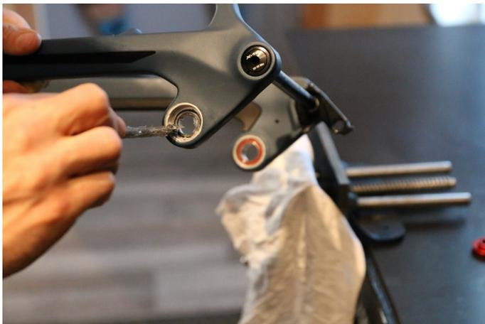
**Step 20:** Press the outer seat stay bearing (6802) into the seat stay. Repeat steps 19-20 on the other side of the seat stay.
