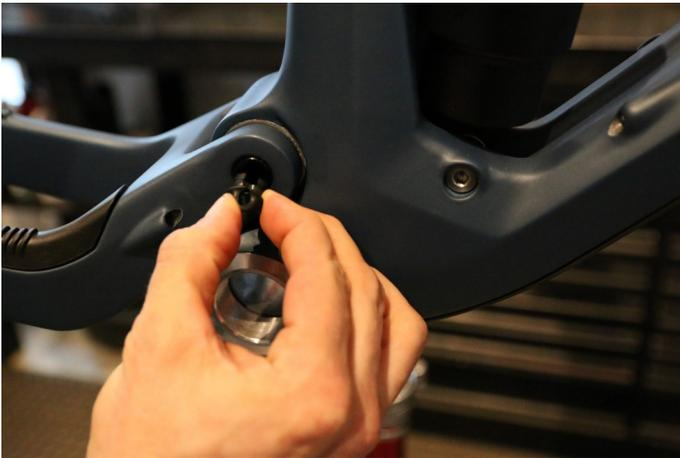
**Step 6:** Remove the main pivot screw with a 5mm allen wrench, make sure you have the washer. Then remove pivot taper nut. If it doesn't come out you can use a 6mm allen wrench to back it out. See photo for orientation.
